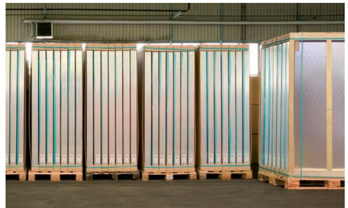
**Packaging** The solar panels are packed vertically on pallets to optimize storage and transportation costs.
